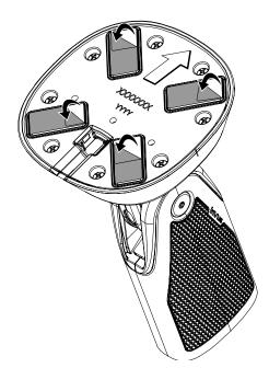
9 Center the top of the handle onto the back of the tablet and apply pressure for at least 10 seconds.
