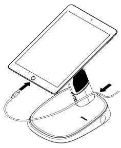
Plug the OEM power supply into the
