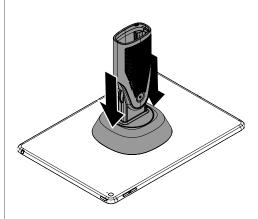
Place the handle and tablet onto the stand.
