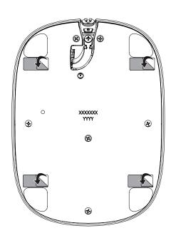
Place the stand in the desired location on the surface and apply pressure for at least 10 seconds.
