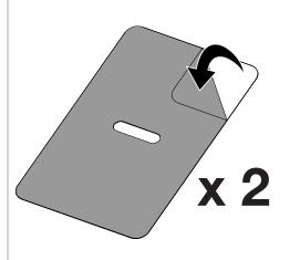
7b Center the 2 LSE plates, adhesive side down, onto the back of the device. Apply pressure for at least 10 seconds.
