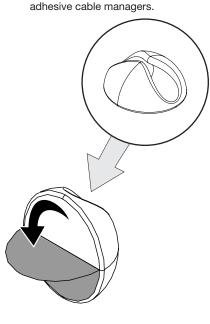
Place the OEM power cable into the cable managers. Place the adhesive cable managers <u>where desired</u> and apply pressure for at least 10 seconds.
